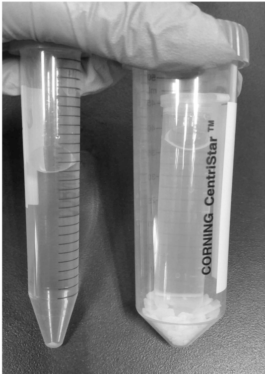
图 1 染色防污染存储(左:醋酸铀染液存储于 15 mL 离心管;右:柠檬酸铅染液存储于 10 mL 离心管,并置于含固体 NaOH 的 50 mL 离心管中)。 Fig. 1 The storage of dye liquor. Left: uranyl acetate stored in 15 mL centrifuge tube. Right: lead citrate stored in 10 mL centrifuge tube which was put in 50 mL centrifuge tube containing NaOH.
